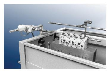
For the small shop with limited requirements, mandrels may be special ordered to allow honing various O.H.C. cylinder heads. Contact Customer Service for details and information. Pictured is a cylinder head being honed on CH-100 Honing Machine with a hand fed Porta-Hone.
