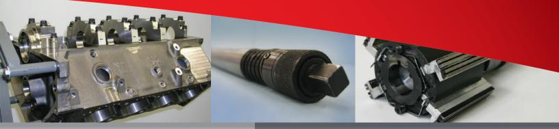
If you put in a reground crankshaft and new inserts without an align hone job ... you'll wind up with crankshaft bind. This robs the engine of horsepower and causes new inserts to wear quickly. Or, excessive cap stretch reduces bearing crush (which holds the insert in place), causing the insert to seize and spin. This results in a scored main bearing bore housing and often a broken crankshaft.
